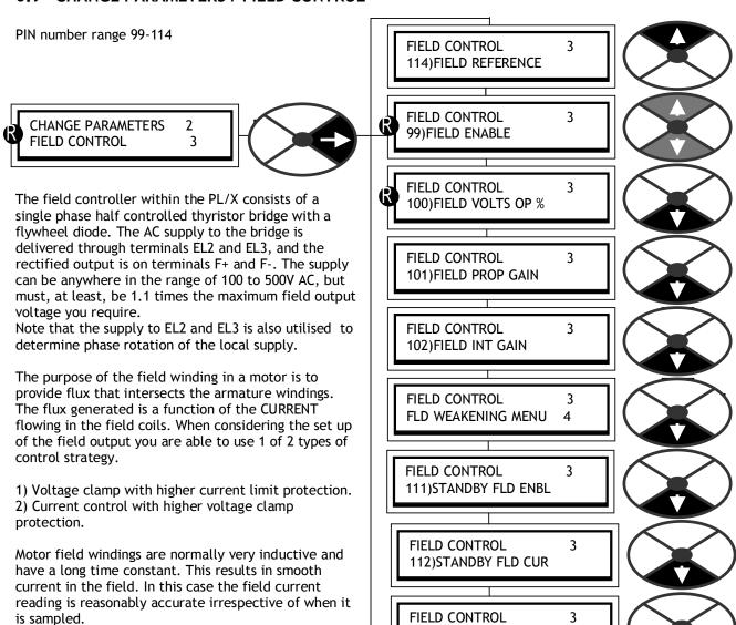
Some motors have shorter field winding time constants than normal resulting in up to 20% ripple. In
