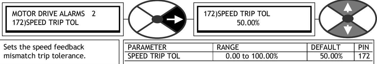
Sets the speed feedback mismatch trip tolerance.
