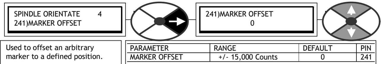
Used to offset an arbitrary marker to a defined position.
