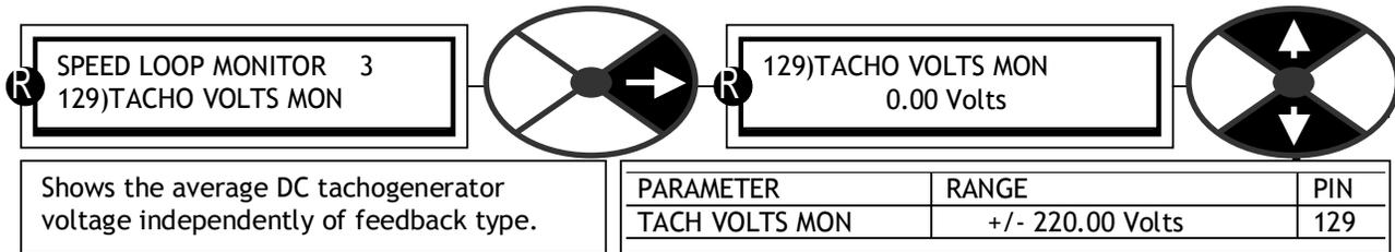
Shows the average DC tachogenerator voltage independently of feedback type.
