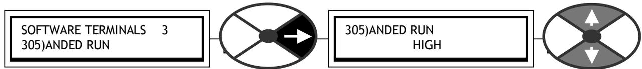
Sets a logic input to an internal AND gate to control RUN.
