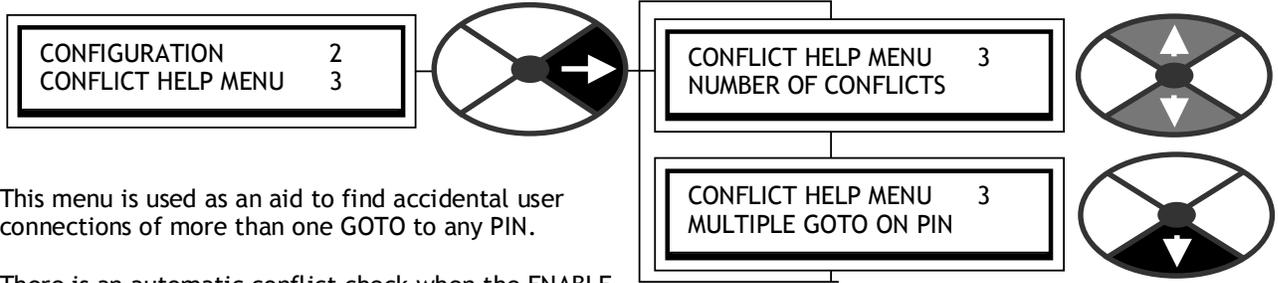
This menu is used as an aid to find accidental user connections of more than one GOTO to any PIN.
