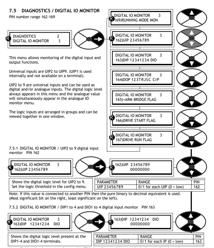
Note. If this value is connected to another PIN then the pure binary to decimal equivalent is used. (Most significant bit on the right, least significant on the left).
