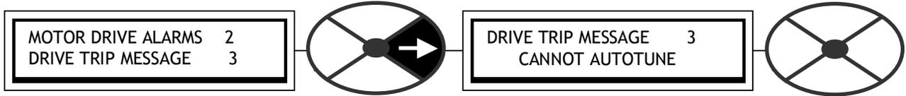
During autotune the drive turns off the field to prevent shaft rotation. An "autotune error" will be triggered by speed feedback being > 20% of rated speed or field current feedback being > 5 % of rated field current during the autotune activity.
