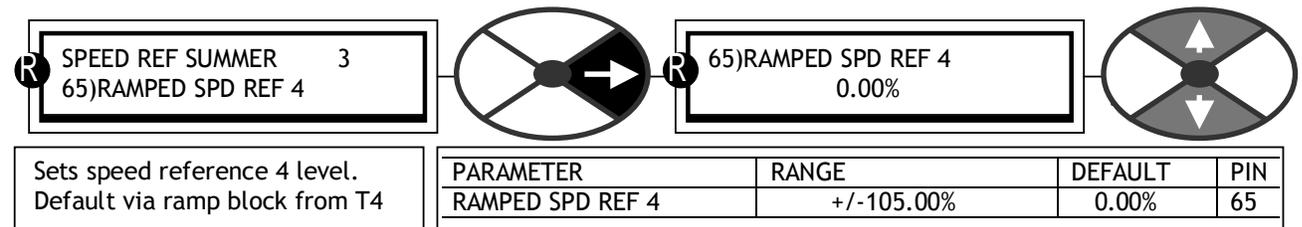
The factory default is to the run mode ramp block output, so this behaves as a monitor for this value.
