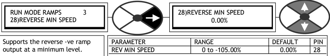
Note that when the FORWARD MIN SPEED parameter (see above) is set between 0 and +0.5%, then the ramp output follows the input at the desired ramp rates through zero, i.e. there are no min speeds operating and there is no hysteresis around zero.
