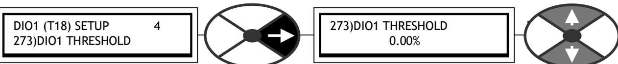
Sets the comparator threshold for the DIOX OP generator.
