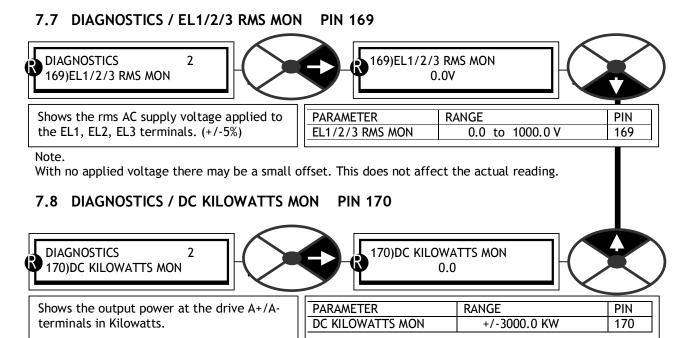
Note. A negative output power shows that the PL/X is regenerating into the AC supply. The power available at the motor shaft will depend on the motor efficiency. (Typically 90 to 95%). To convert Kilowatts to Horsepower multiply by a scaling factor of 1.34.
