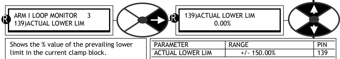
The lowest of all clamps is the prevailing source. See 6.8.1 CURRENT CONTROL / Block diagram.
