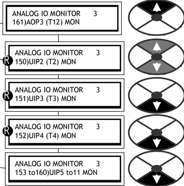
The PL/X possesses a very useful commissioning tool, 260)SCOPE OP SELECT. When enabled, this automatically configures AOP3 on terminal 12 as an oscilloscope probe output. See 13.5.3 ANALOG OUTPUTS / Scope output select PIN 260. The output is automatically connected to whatever parameter is being displayed, and reconnected to its original source after the function is no longer enabled.
