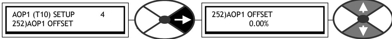
Sets the level of bi-polar offset to be added to the final signal.
