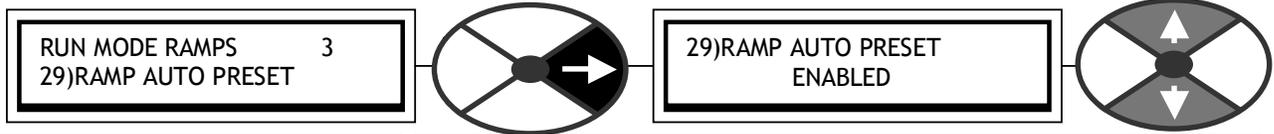
When enabled, the system reset also presets the ramp.
