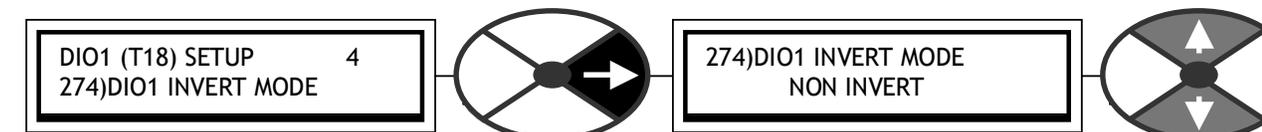
Allows the comparator output logic to be inverted for DIOX.
