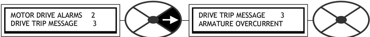
An armature current trip is provided. This is set to operate for current feedback values exceeding 170% of the maximum model current, or 300% of 2)RATED ARM AMPS, whichever is reached first.
