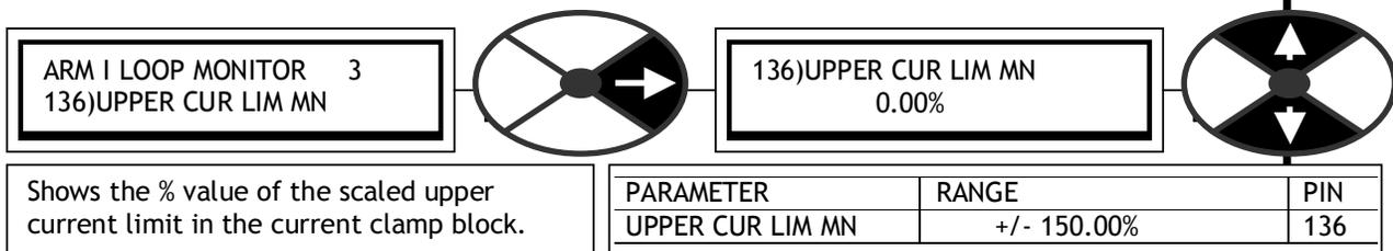
Shows the % value of the scaled upper current limit in the current clamp block.
