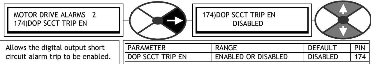
Allows the digital output short circuit alarm trip to be enabled.
