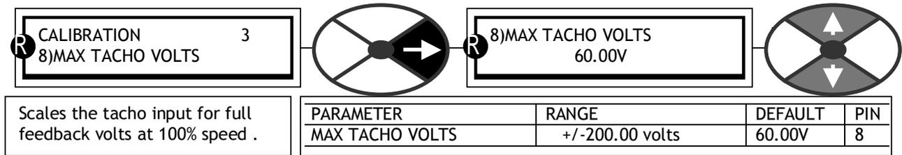
Multiply the output volts per rev value for the tacho by the full speed rpm of the tacho
