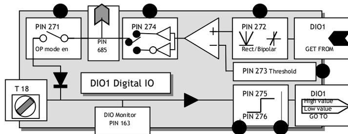
13.7.1.3 DIOX SETUP / DIO1/2/3/4 OP comp threshold PINs 273 / 279 / 285 / 290
