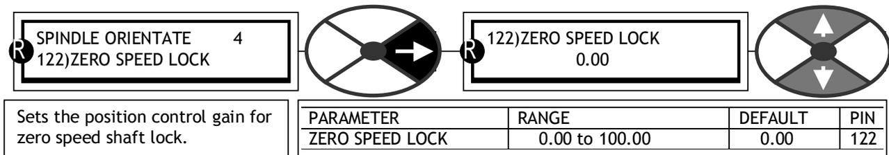
Sets the position control gain for zero speed shaft lock.
