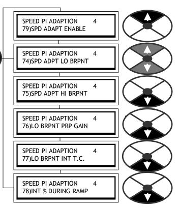
There is also the ability to prevent the integrator from accumulating error during a long speed up ramp. This can be useful for systems involving high inertias where there is a possibility of speed error at the top of the ramp while the loop removes the integrator error. See 6.2.16 RUN MODE RAMPS / Ramping flag PIN 35. See 6.7.7.7 SPEED PI ADAPTION / Using small speed inputs. The default gives low gain for small inputs.
