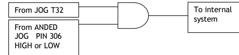
306)ANDED JOG is normally used by a serial link to control the drive. The local hardware terminal in the LOW position will defeat the serial link. The serial link in the OFF position will defeat the local hardware terminal.
