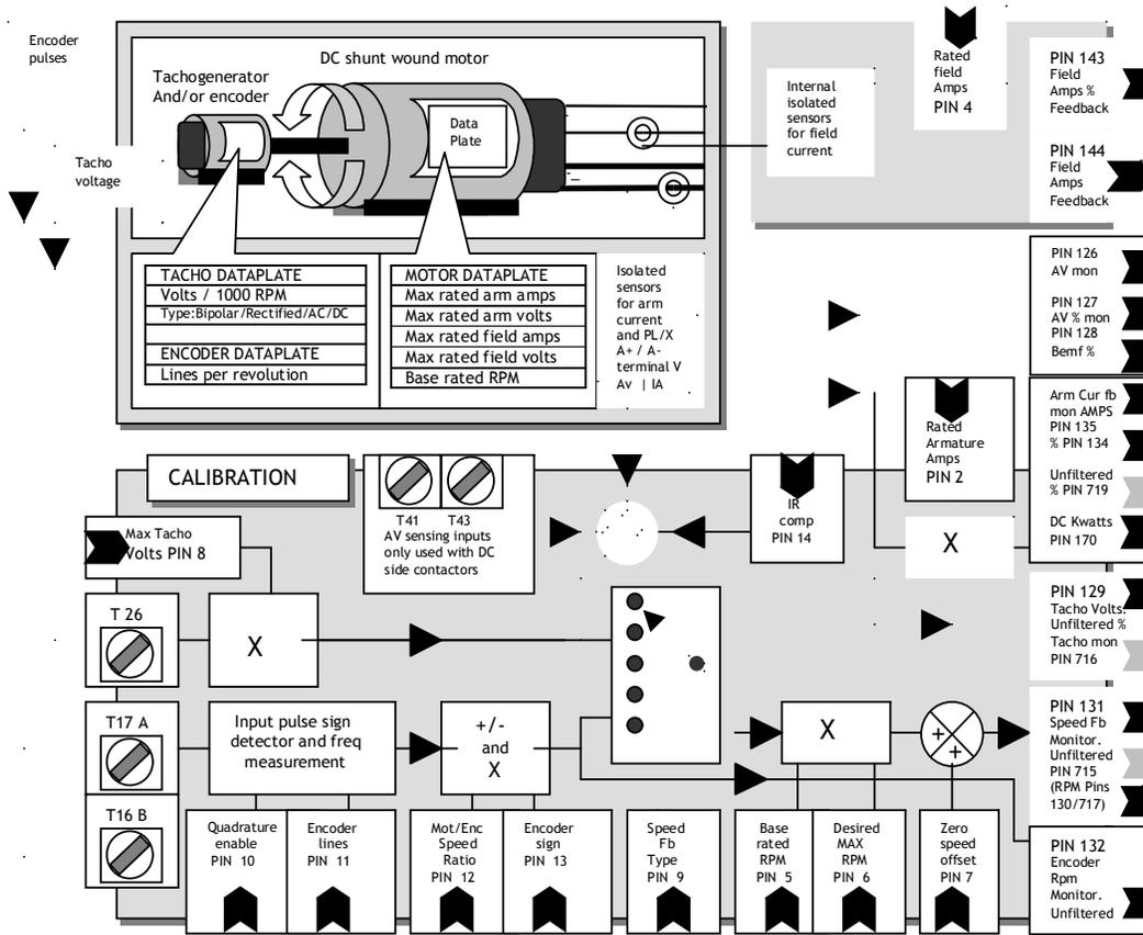
6.1.2 CALIBRATION / Rated armature amps PIN 2 QUICK START
