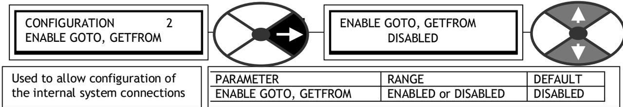
Note. To start a connection configuration session ENABLE GOTO, GETFROM must be set to ENABLED.
