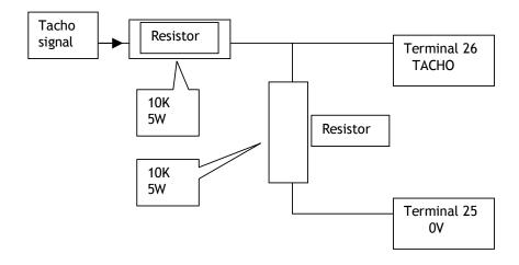
The network shown will allow full scale voltages up to 400 Volts. The number scrolled in the window should be set to half the full scale tacho volts. Appropriate measures must be taken to dissipate the heat from the dropper resistors. The total power in watts dissipated will be (Tacho signal volts)<sup>2</sup> / 20,000.
