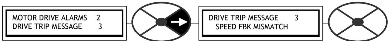
See 8.1.1 MOTOR DRIVE ALARMS / Speed feedback mismatch trip enable PIN 171.
