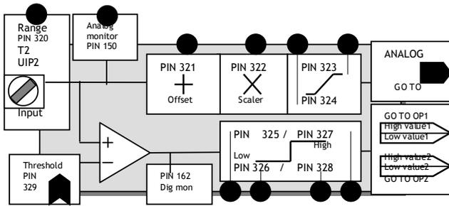
There are 2 independent digital outputs driven by the comparator. Each has a GO TO connection plus a value for high and a value for low.
