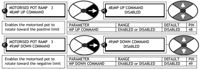
Default connections to terminal 8 (Up) and terminal 9 (Down). Note. There is no ramping with Up and Down enabled together.
