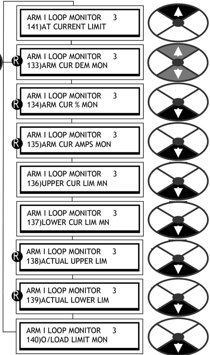
7.2.1 ARM I LOOP MONITOR / Armature current demand monitor PIN 133
