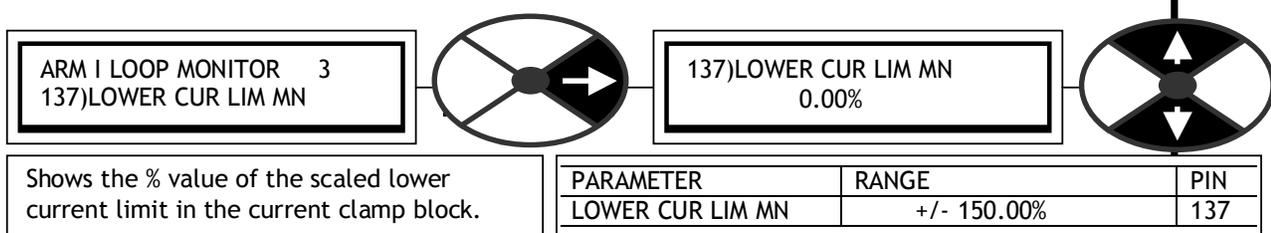
Shows the % value of the scaled lower current limit in the current clamp block.
