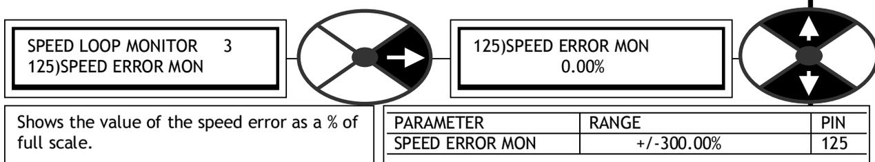
7.1.4 SPEED LOOP MONITOR / Armature volts monitor PIN 126
