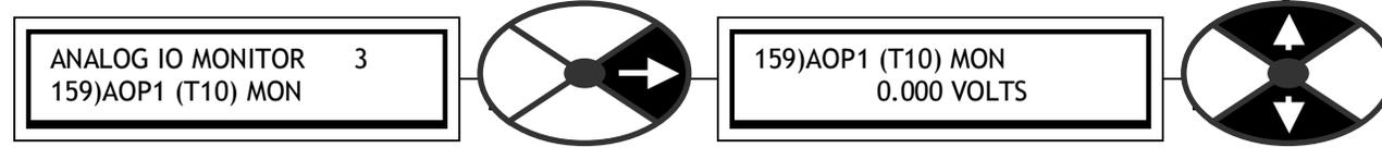
Shows the analogue output voltage for AOP1/2/3 (PIN numbers 159, 160, 161)
