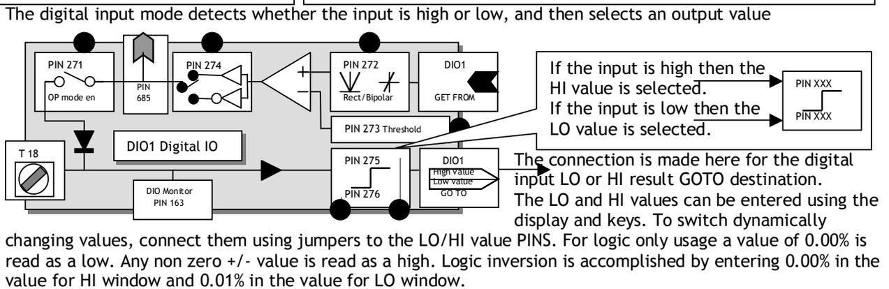
13.7.1.7 DIOX SETUP / DIO1/2/3/4 Input high value PINs 275 / 281 / 287 / 293
