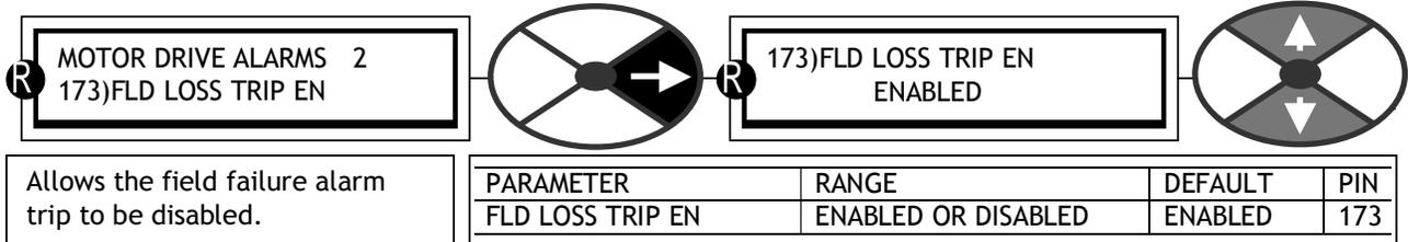
Allows the field failure alarm trip to be disabled.
