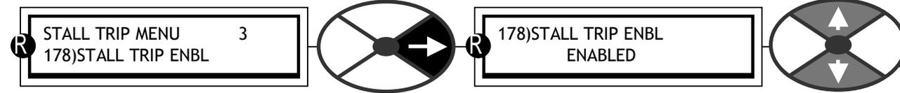
Allows the motor stall alarm trip to be enabled.
