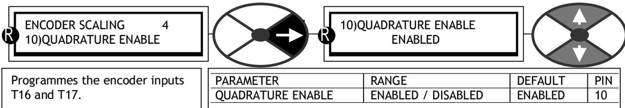
The encoder inputs on T16 and T17 can be programmed to accept 2 types of encoder pulse trains.
