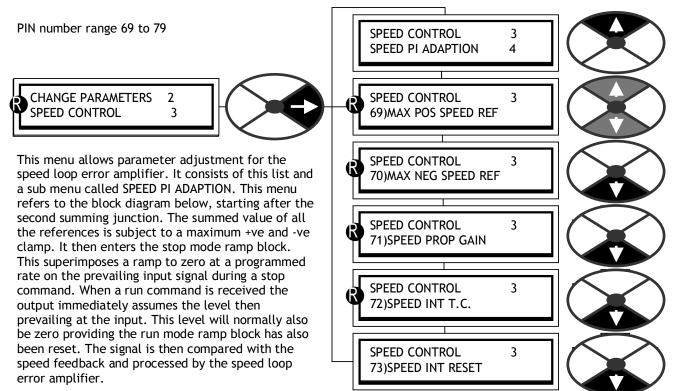
The basic PI gain and time constants are adjustable in this list, and with further sophistication in the sub list SPEED PI ADAPTION. After being output from the error amplifier the signal now represents current reference. This current reference signal is then selected for output by the speed bypass change over switch. If the speed bypass mode is enabled then input reference 3 is selected.
