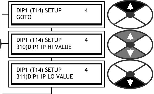
13.6.2.1 DIPX SETUP / DIP1/2/3/4 Input high value PINs 310 / 312 / 314 / 316
