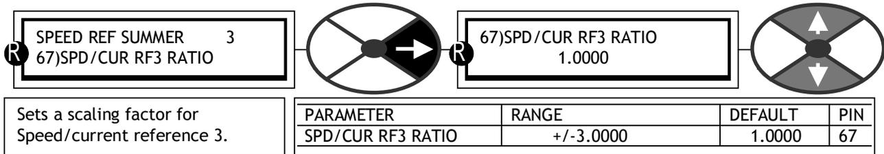
Sets a scaling factor for Speed/current reference 3.
