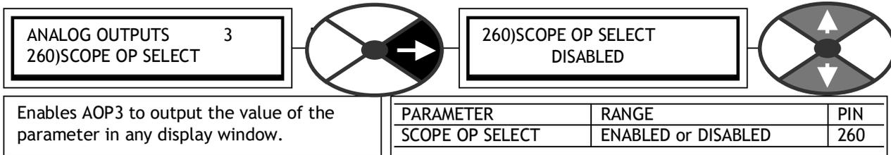
Enables AOP3 to output the value of the parameter in any display window.
