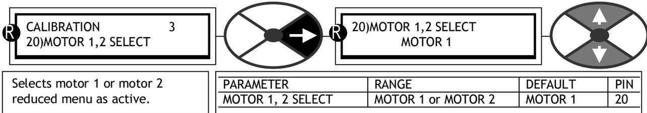
All the alterable parameters contained in the CHANGE PARAMETERS reduced menu may have 2 value settings. (MOTOR 1 and MOTOR 2). This window selects the active set. The active set is always the one available in the CHANGE PARAMETERS menu display. The passive set can be viewed and modified in the configuration menu. See 13.14.1 DRIVE PERSONALITY / PASSIVE MOTOR SET.
