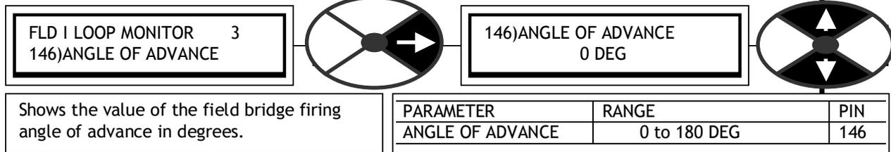
Shows the value of the field bridge firing angle of advance in degrees.
