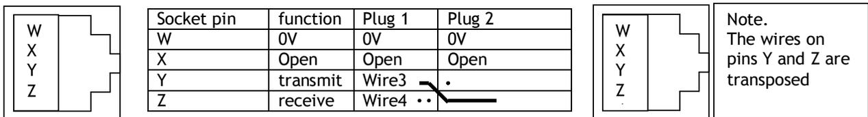
(Unit to unit 2 metre cable part number LA102596. Unit to host, 9 way female Dtype part no. LA102595).
