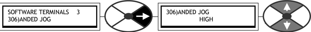
Sets a logic input to an internal AND gate to control JOG
