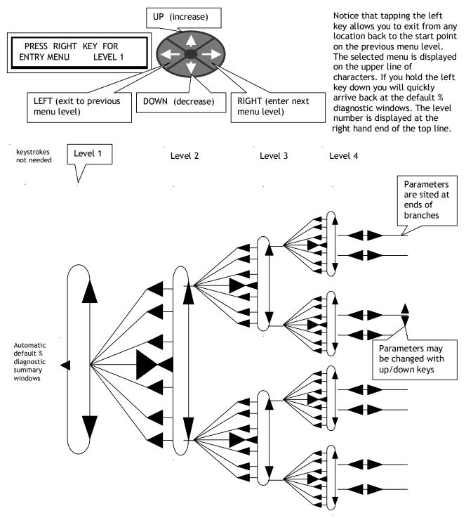
As well as travelling around the tree structure the keys perform other functions. These are as follows.
