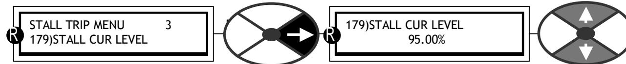
Sets the stall alarm trip LEVEL as a % of rated motor amps.
