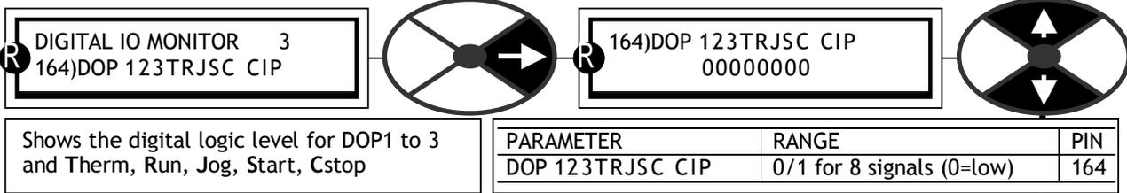
Shows the digital logic level for DOP1 to 3 and Therm, Run, Jog, Start, Cstop
