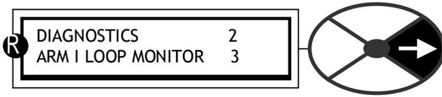
This menu allows monitoring of the parameters associated with the inputs to the current loop.
