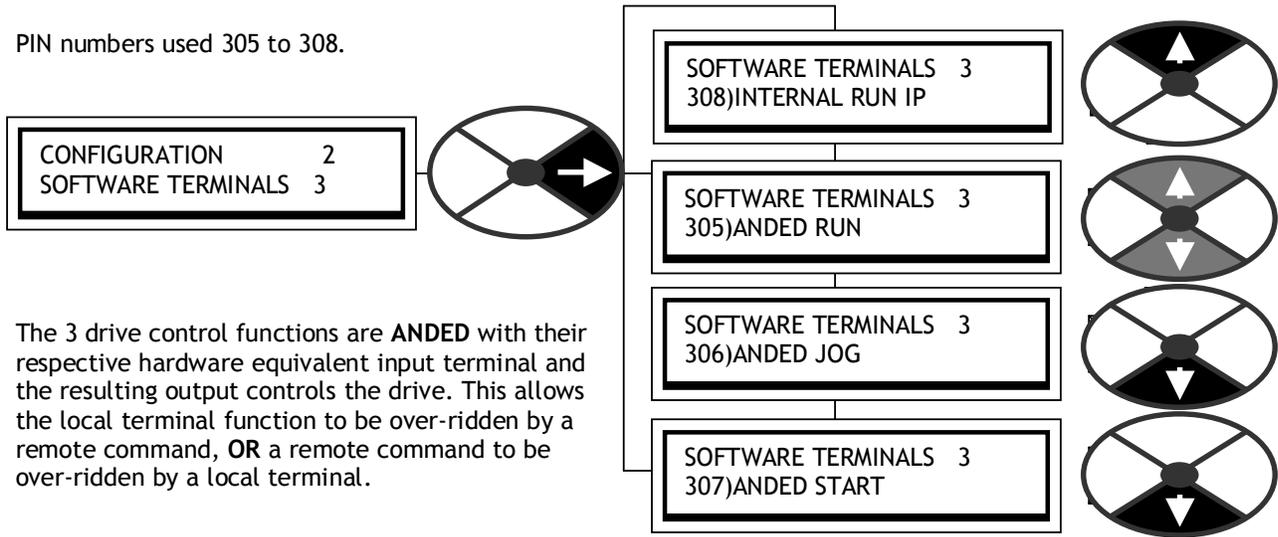
The 3 drive control functions are **ANDED** with their respective hardware equivalent input terminal and the resulting output controls the drive. This allows the local terminal function to be over-riden by a remote command, **OR** a remote command to be over-riden by a local terminal.
