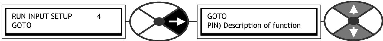
Defines the target PIN for the connection to RUN IP
