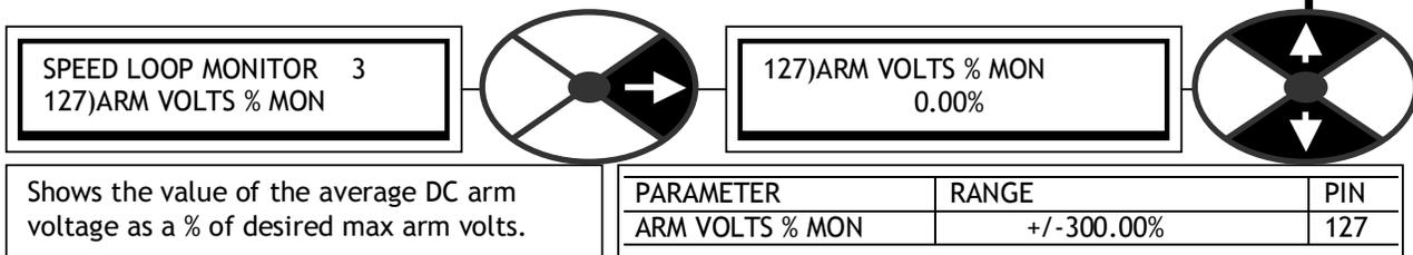
Note. The 100% level is equivalent to 18)RATED ARM VOLTS
