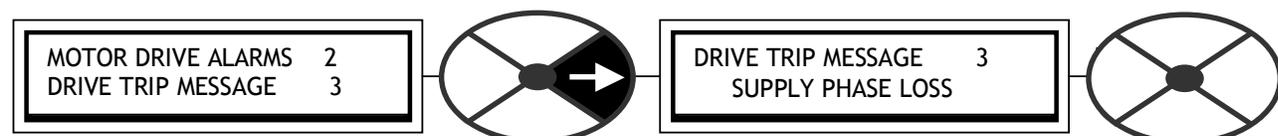
The controller continuously monitors the incoming supply of the EL1, EL2 connections. If either are lost, the alarm will operate. The subsequent control action depends on the running condition at the time the alarm is triggered. The message will also briefly appear after the control supply has been removed.
