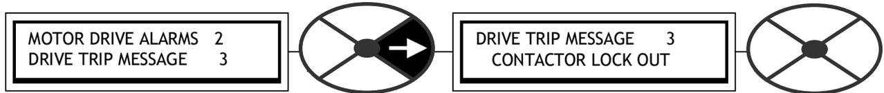
This alarm may be caused by two possible events at the commencement of a running mode request. It is accompanied by automatic inhibiting of the current loop followed by de-energisation of the contactor.
