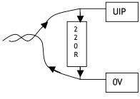
When using 4-20mA loop signals all that is required is to fit an external burden resistor of 220 Ohms between the input and 0V. The resulting voltage signal generated by passing the signal current through the burden will be +0.88V for 4 mA (represents 0%) and 4.4V for 20mA (represents 100%). Using the appropriate UIPX SETUP block, select the following:-
