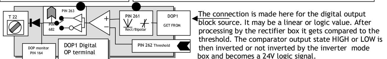
For comparing logic values always put 0.00% in the threshold window. The comparator output is low for identical inputs.
