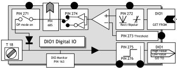
The connection is made here for the digital output block source. It may be a linear or logic value. After processing by the rectifier box it gets compared to the threshold. The comparator output state HIGH or LOW is then inverted or not inverted by the inverter mode box. It then proceeds to the output stage through the digital output enable switch and becomes a 24V logic signal. It is also available for internal
