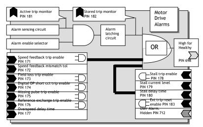
If an alarm is enabled, triggered and latched causing the drive to shut down, then after approximately a further 10mS no further alarms will be latched. Hence when the latched status of the alarms is monitored it is unlikely that more than 1 alarm will be latched. If however more than 1 is latched, then the first that arrived and initiated the shutdown can be determined from the DRIVE TRIP MESSAGE menu.
