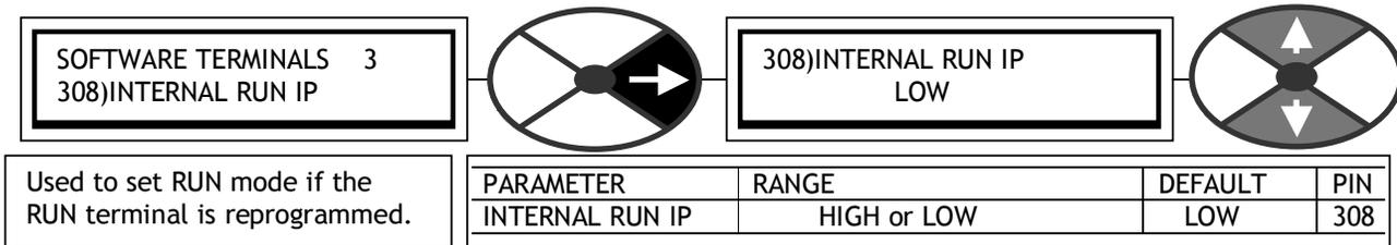
The RUN command normally comes from the default RUN terminal (T31) and will show the state of T31. However this terminal may be used as a programmable terminal in the event of a shortage of digital inputs. In this case 308)INTERNAL RUN IP must be disconnected from the RUN terminal and set HIGH to allow the drive to run.
