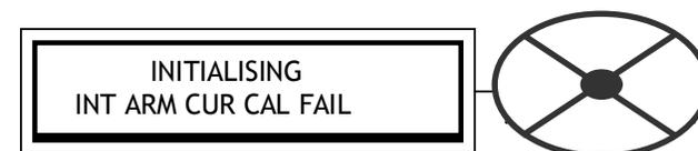
9.1.6 SELF TEST MESSAGE / Stop drive to adjust parameter
