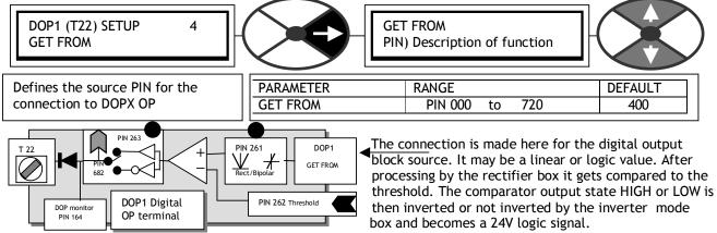
For comparing logic values always put 0.00% in the threshold window. The comparator output is low for identical inputs.
