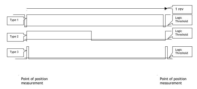
Type 1 is the preferred marker signal. This is because for most of the time the signal is well away from the logic threshold and noise is very unlikely to cause a false marker reading.
