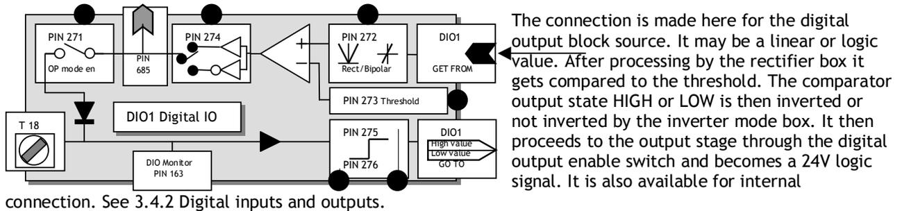
13.7.1.6 DIOX SETUP / DIO1/2/3/4 Make input GOTO destination connection
