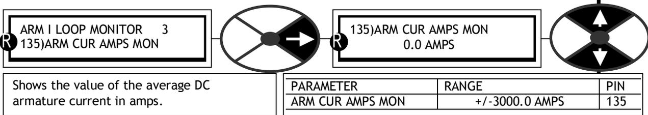
Shows the value of the average DC armature current in amps.
