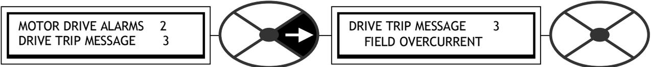
The controller checks that the field current does not exceed 115% of 4)RATED FIELD AMPS.
