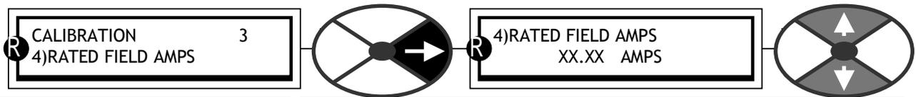
This is the desired 100% DC output field current in amps
