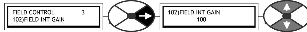
Sets the integral gain of the field current control loop.
