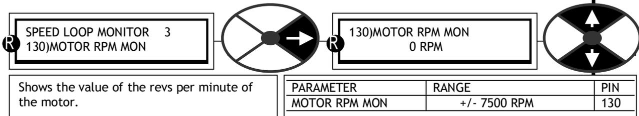
Shows the value of the revs per minute of the motor.
