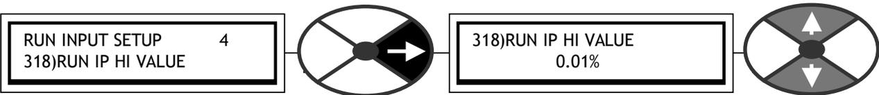
Sets the level of the value selected by a high RUN input.
