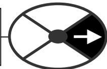
4) Select the quick start parameters by using the up / down keys. Press the right key to enter the parameter adjustment window for each in turn. Modify each one to suit your system using the up/down keys. Use the left key to back out of each parameter adjustment window and return to the circular CALIBRATION menu.
