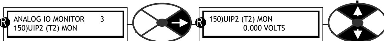
Shows the analogue voltage for the universal inputs 2 to 9.
