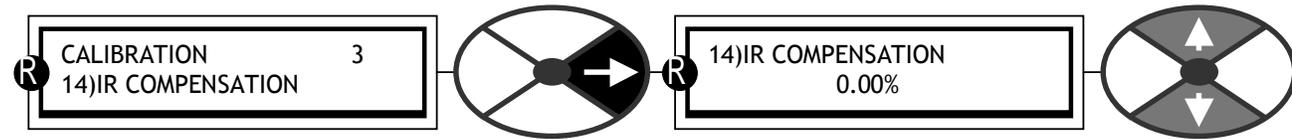
Sets % compensation of the AVF signal due to IR drop
