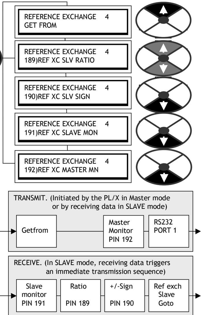
**Multi Drive Digital speed locking.** Daisy chain using reference exchange and encoder feedback for each drive. When using this for digital speed accuracy, it is important that the remaining analogue inputs do not inject small errors into the loop when they are dormant. See 6.7 CHANGE PARAMETERS / SPEED CONTROL. Useful tips for eliminating unwanted analogue references.
