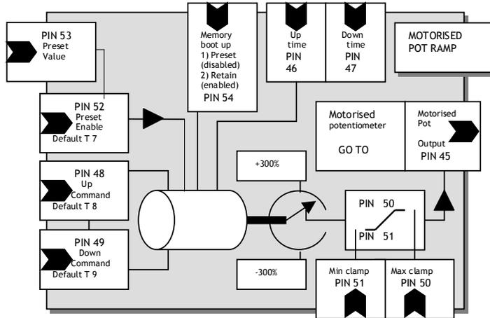
6.4.2 MOTORISED POT RAMP / MP output monitor PIN 45
