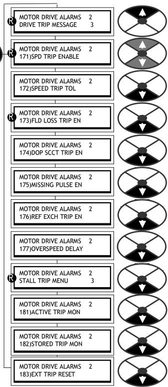
alarms. The quoted times are typical since the delay is implemented in microprocessor "cycle time" units which vary with microprocessor loading. The arrival of the alarms prior to the trigger can be accessed for advance warning purposes using the active monitor window. There is a USER ALARM on hidden PIN 712. This may be connected by the user to any flag, to trip the drive.
