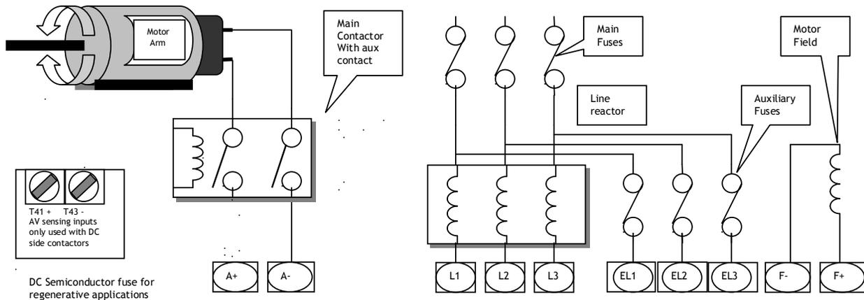
Wire the auxiliary N/O contact in series with RUN (T31) and +24V (T35)
