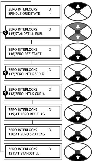
**ii)** 116)ZERO REF START. This prevents the current control being enabled after a start command, if the total speed reference to the drive, or the input to the RUN MODE RAMPS, is not at zero. It is used if starting the motor inadvertently may be undesirable. The message CONTACTOR LOCK OUT will appear after approximately 2 seconds if this function is not satisfied. The contactor is de-energised.
