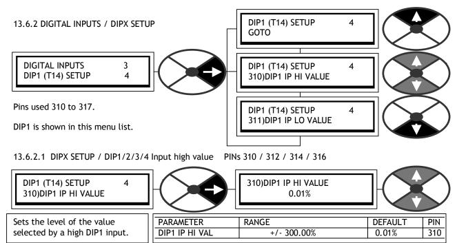
Note. You can make a simple AND gate by selecting this as the target PIN of a logical GOTO.
