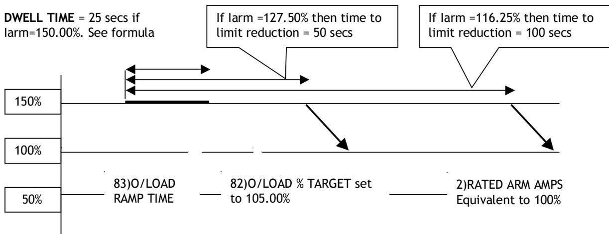
Formula for calculating Dwell time for a given PIN82 Overload % target and PIN138 prevailing Current Limit%
