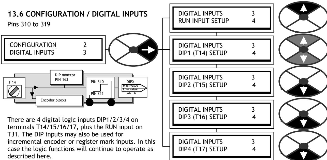
There are 4 digital logic inputs DIP1/2/3/4 on terminals T14/15/16/17, plus the RUN input on T31. The DIP inputs may also be used for incremental encoder or register mark inputs. In this case the logic functions will continue to operate as described here.
