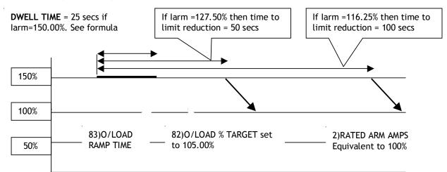
Formula for calculating Dwell time for a given PIN82 Overload % target and PIN138 prevailing Current Limit% DWELL TIME = (150%-PIN82%) x 25/(I limit%-PIN82%) in seconds. (Assuming current remains at the limit).
