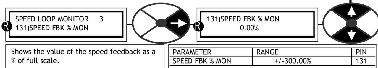
Shows the value of the speed feedback as a % of full scale.
