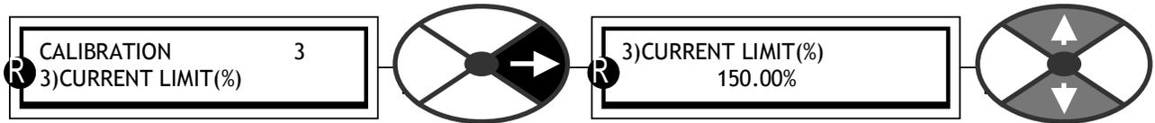
This is the desired current limit % of 2)RATED ARM AMPS
