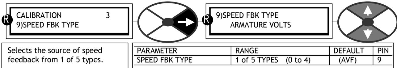
The speed feedback can be derived from 1 of 3 fundamental sources or a combination of them.
