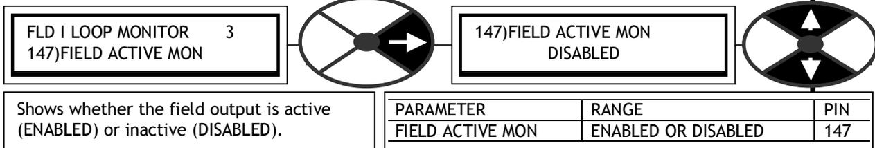
Shows whether the field output is active (ENABLED) or inactive (DISABLED).
