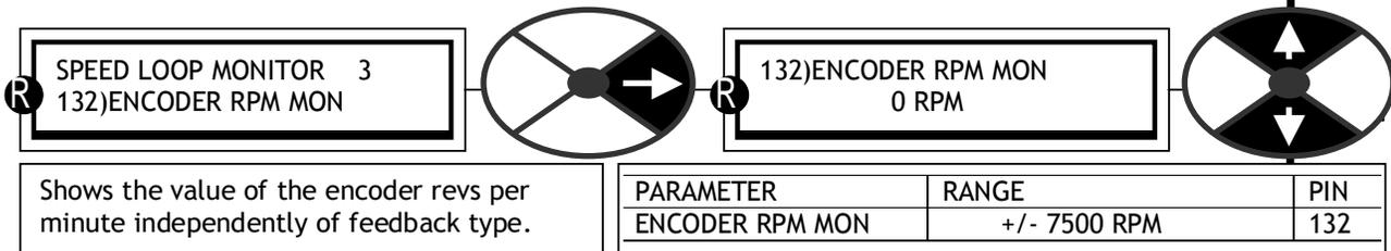
Shows the value of the encoder revs per minute independently of feedback type.
