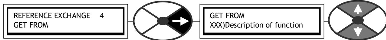
Defines the source PIN for data to output via the TRANSMIT channel
