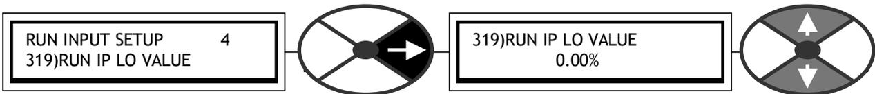
Sets the level of the value selected by a low RUN input.
