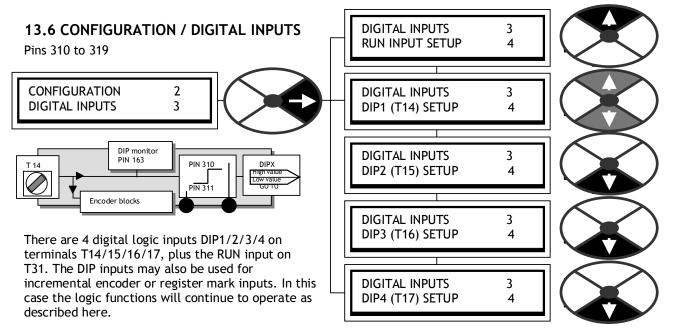
The LO and HI values can be entered using the display and keys, or may be connected to other output PINs using JUMPERS. This turns the function into a change-over switch for dynamic values. For logic only usage a value of 0.00% is read as a low. Any non zero +/- value is read as a high. Logic inversion is accomplished by entering 0.00% in the value for HI window and 0.01% in the value for LO window.
