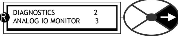
Analogue inputs are UIP2 to UIP9. The UIP number corresponds to its terminal number. (UIP1 is used internally and not available on a terminal). UIP2 to 9 are universal inputs and can be used as digital and/or analogue inputs. The analogue value appears in this menu and the digital logic level will simultaneously appear in the digital IO menu.
