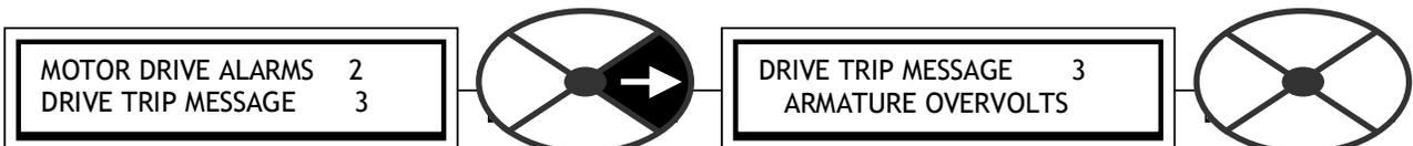
If the motor armature voltage feedback exceeds 18)RATED ARM VOLTS by more than 20% then this alarm will operate. . 18)RATED ARM VOLTS may be lower than the dataplate maximum. This alarm operates with any source of speed feedback.
