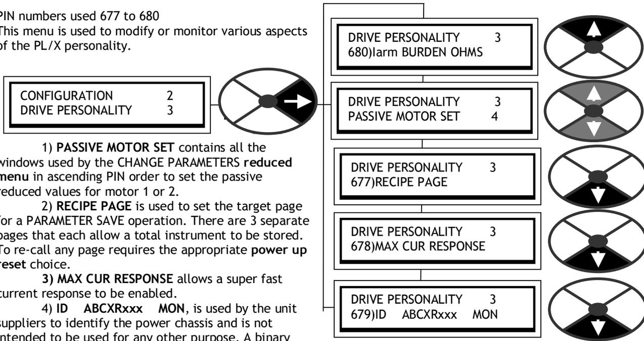
1) **PASSIVE MOTOR SET** contains all the windows used by the **CHANGE PARAMETERS reduced menu** in ascending PIN order to set the passive reduced values for motor 1 or 2.
