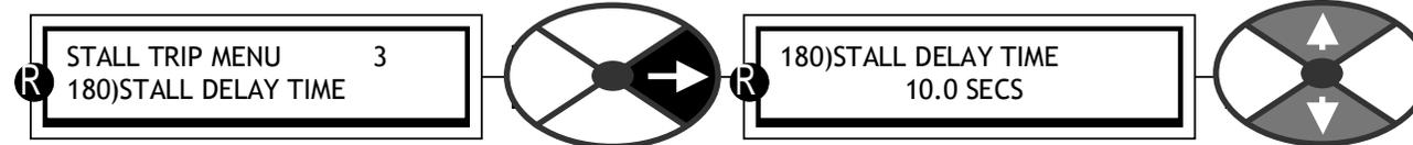
Sets the delay time between stall start and alarm trigger.
