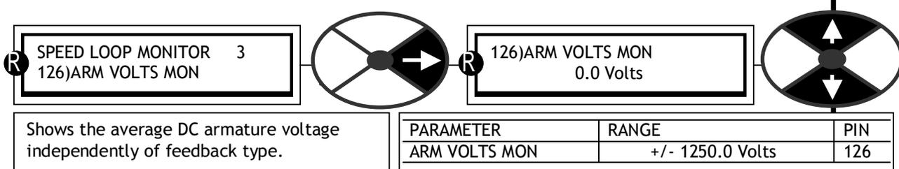
7.1.5 SPEED LOOP MONITOR / Armature volts % monitor PIN 127
