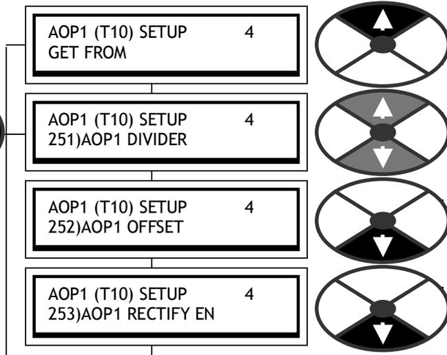
13.5.2.1 AOPX SETUP / AOP1/2/3 Dividing factor PINs 251 / 254 / 257
