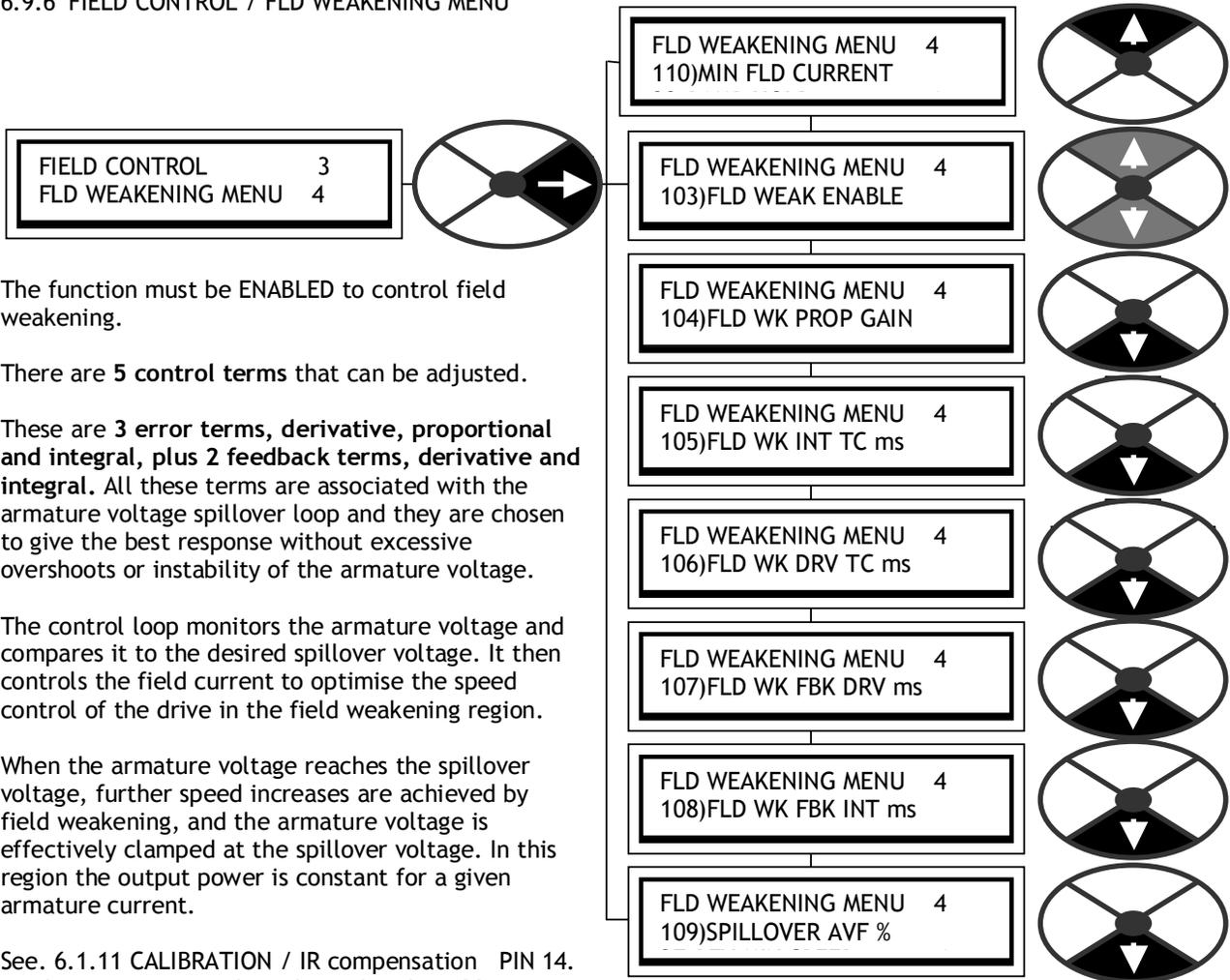
The function must be ENABLED to control field weakening.
