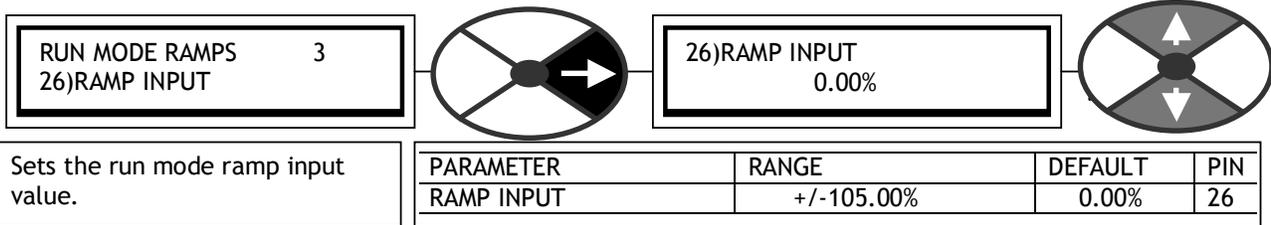
The factory default connects T4 to PIN 26. This allows an external analogue reference to enter the ramp input value, and then this parameter behaves as a monitor of the ramp input value.
