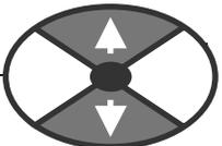
Enables the motorised pot to rotate toward the positive limit
