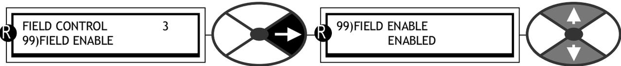
This allows the field output to be enabled or disabled.
