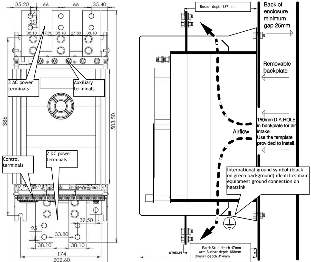
The units must be orientated vertically as shown.
