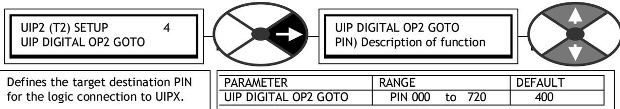
All UIP DIGITAL OP2 GOTO default connections are 400)Block Disconnect.
