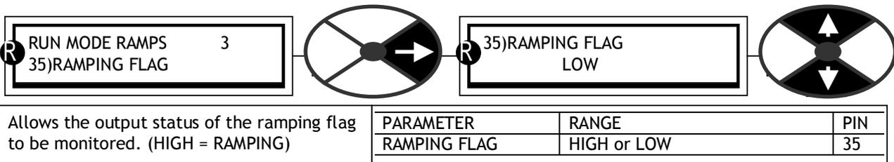
The ramping flag may be used to modify the speed loop integrator during ramping. See 6.7.7.5 SPEED PI ADAPTION / Integral % during ramp PIN 78. Note. 78)INT % DURING RAMP does not reset the integrator, it merely alters the % of integration.
