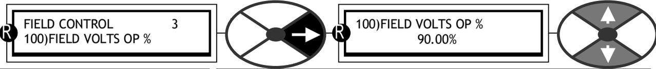
Sets the DC field voltage clamp as a % of the AC supply volts.
