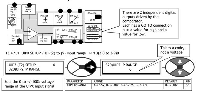
The  $\pm$ -5V and  $\pm$ -10V ranges are the most accurate (0.4%, typically 0.1%).
