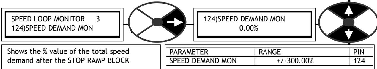
7.1.3 SPEED LOOP MONITOR / Speed error monitor PIN 125
