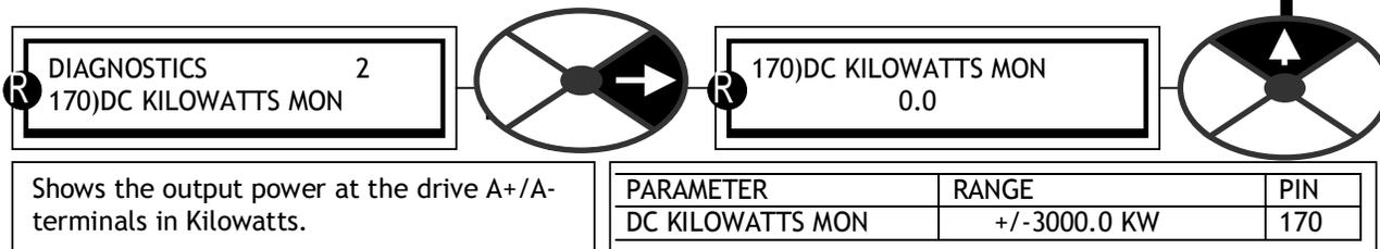
Note. A negative output power shows that the PL/X is regenerating into the AC supply. The power available at the motor shaft will depend on the motor efficiency. (Typically 90 to 95%). To convert Kilowatts to Horsepower multiply by a scaling factor of 1.34.
