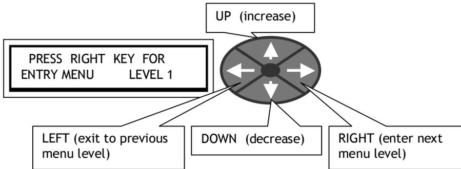
Notice that tapping the left key allows you to exit from any location back to the start point on the previous menu level. The selected menu is displayed on the upper line of characters. If you hold the left key down you will quickly arrive back at the default % diagnostic windows. The level number is displayed at the right hand end of the top line.
