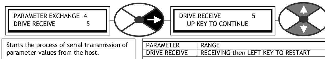
See 10.2.4 Rules of parameter exchange relating to software version. See also 5.3 Archiving PL/X recipes. This is the transfer of the Parameters from the host to the PL/X. This information is written directly to the drive's permanent memory, so **the drive's present settings for the TARGET RECIPE PAGE will be overwritten.** The file will contain its recipe page source (Normal, 2, 3) and will automatically save on that recipe page. See also. 10.2.1.1 PARAMETER EXCHANGE with a locked recipe page 3
