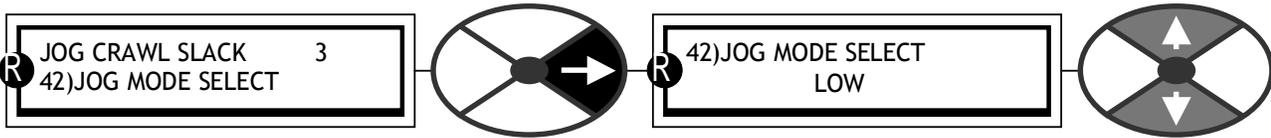
Combines with the JOG/START inputs for jog/crawl/slack mode
