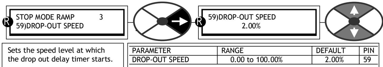
Sets the speed level at which the drop out delay timer starts.
