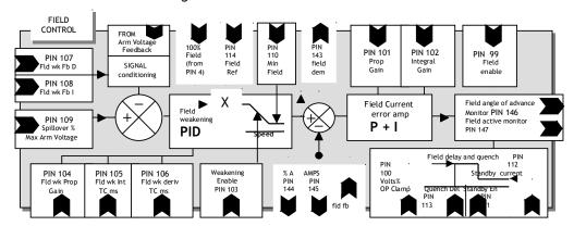
1) Voltage output clamp. This is an open loop setting of the field bridge-firing angle allowing the DC output voltage to be set between 0 to 90% of the incoming supply voltage. E. g. for an AC supply of 400V the 90% output voltage is 360V DC. Note if the AC supply varies, then the field output voltage will vary in proportion. Also if the field resistance changes then the resulting output current will change.
