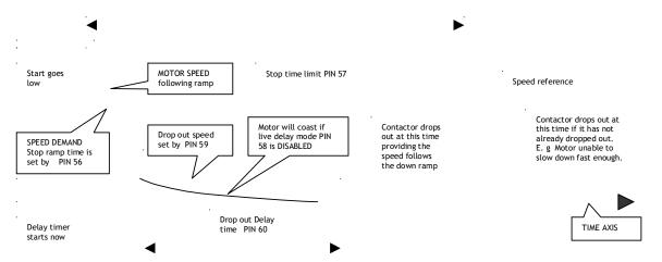
If START or JOG goes high during the 60)DROP-OUT DELAY time, then the contactor stays energised and the drive will restart immediately. The 60)DROP-OUT DELAY timer will be reset to time zero. This allows jogging without the contactor dropping in and out.
