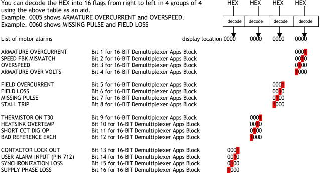
Note. There is an Application Block called 16-DEMULTIPLEX which can extract a flag for each of these Alarms See section 12 APPLICATION BLOCKS and also refer to Part 2 Application Blocks Manual for more detail.
