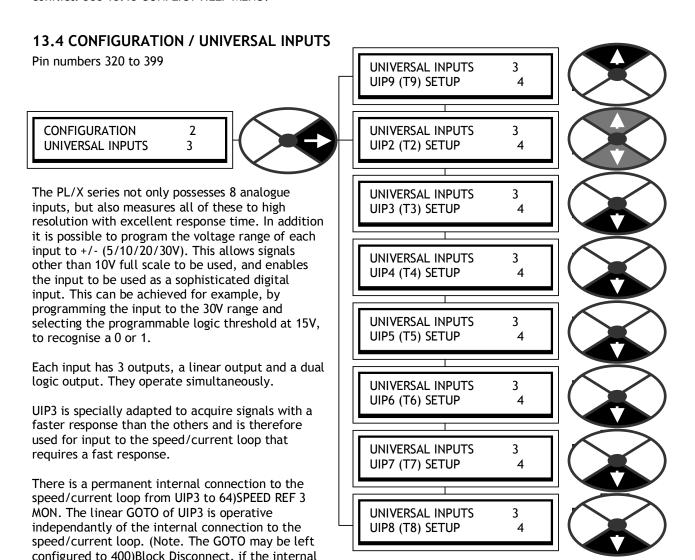
connection is utilised). To connect UIP3 elsewhere, nullify the internal connection, (set 67)SPD/CUR RF3 RATIO in the SPEED REF SUMMER menu to 0.0000), then reconfigure the linear GOTO. The parameter 64)SPEED REF 3 MON is a monitor of the UIP3 analog output.
