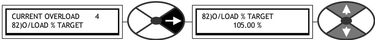
Sets the current limit target level after excessive overload.
