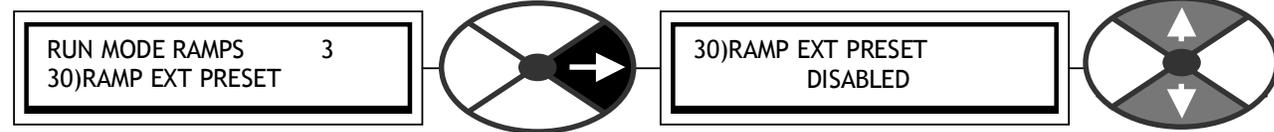
When enabled the ramp is held in preset mode.
