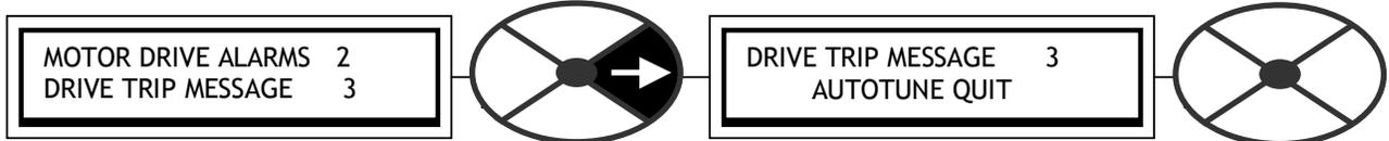
The controller will quit the autotune function if the coast stop, start or run terminals are disabled (taken low) Alternatively, if the autotune ENABLE/DISABLE is instructed to be DISABLED during its autotune sequence then this message will appear. See 6.8.9 CURRENT CONTROL / Autotune enable PIN 92. A time-out ( approx. 2 mins) will also cause an autotune quit.
