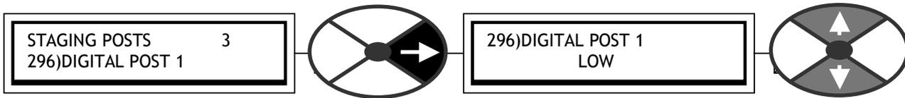
Used as storage point for logic state and/or connecting point.
