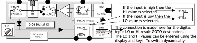
changing values, connect them using jumpers to the LO/HI value PINS. For logic only usage a value of 0.00% is read as a low. Any non zero +/- value is read as a high. Logic inversion is accomplished by entering 0.00% in the value for HI window and 0.01% in the value for LO window.
