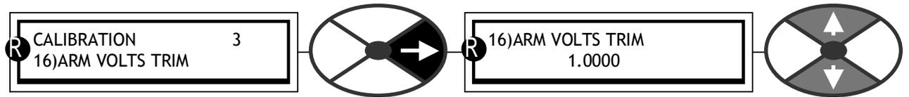
Sets a positive trim factor for the armature volts feedback
