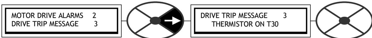
It is good practice to protect DC motors against sustained thermal overloads by fitting temperature sensitive resistors or switches in the field and interpole windings of the machine. Temperature sensitive resistors have a low resistance (typically 200 Ohms) up to a reference temperature (125 deg C). Above this, their resistance rises rapidly to greater than 2000 Ohms.
