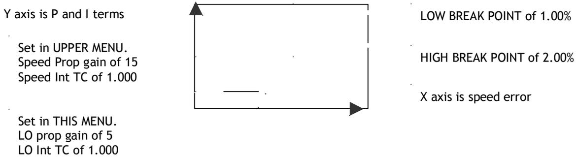
**Note.** The default settings are designed to give lower gain with low error. This provides smooth steady state performance. Applications that require precise control at very low speeds may function better with the adaption disabled.
