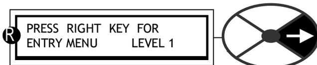
After tapping the right key to proceed to the next level, you can travel up and down the level using the up and down keys. The menus are circular so you can travel up or down to reach your desired destination. The menus are designed so that the most frequently used windows are closest to the entry points.
