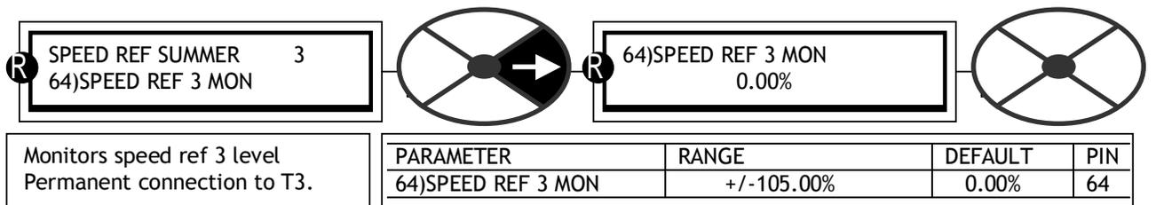
T3 is internally connected via UIP3 to 64)SPEED REF 3 MON, so this behaves as a monitor of T3 IP value. This parameter is not adjustable from the keys. It has the fastest sample rate for rapid response applications. Note. When 97)SPD BYPASS CUR EN is ENABLED this monitor is set to zero. Use 133)ARM CUR DEM MON.
