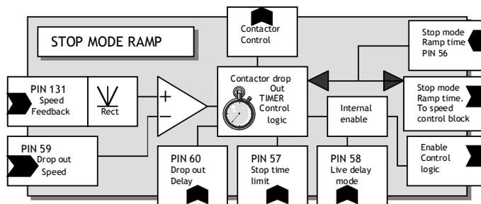
6.5.1.1 Block diagram of contactor control
