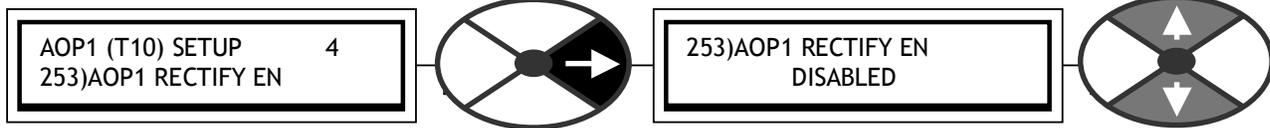
Allows the output mode to be rectified when enabled.
