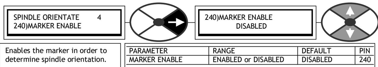
DISABLED turns off the spindle orientate function and the marker frequency monitor function. Note, 122)ZERO SPEED LOCK function will continue to work however stopping position is arbitrary.
