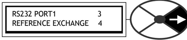
In MASTER mode the unit initiates high bandwidth transmission of data, and can also receive data.
