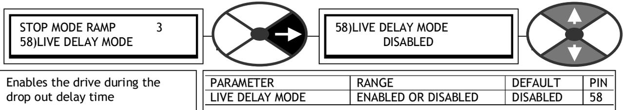
Enables the drive during the drop out delay time
