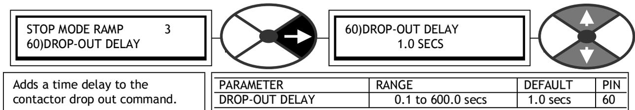
Adds a time delay to the contactor drop out command.
