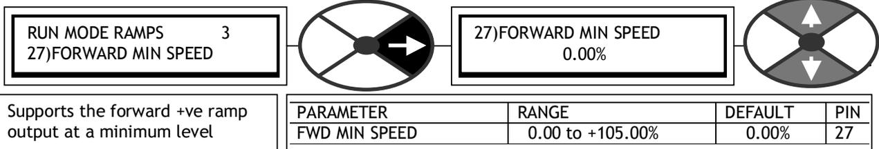
Note that when this parameter is set between 0 and +0.5%, then the ramp output follows the input at the desired ramp rates through zero, i.e. there are no min speeds operating and there is no hysteresis around zero.
