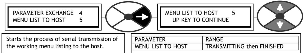
Starts the process of serial transmission of the working menu listing to the host.
