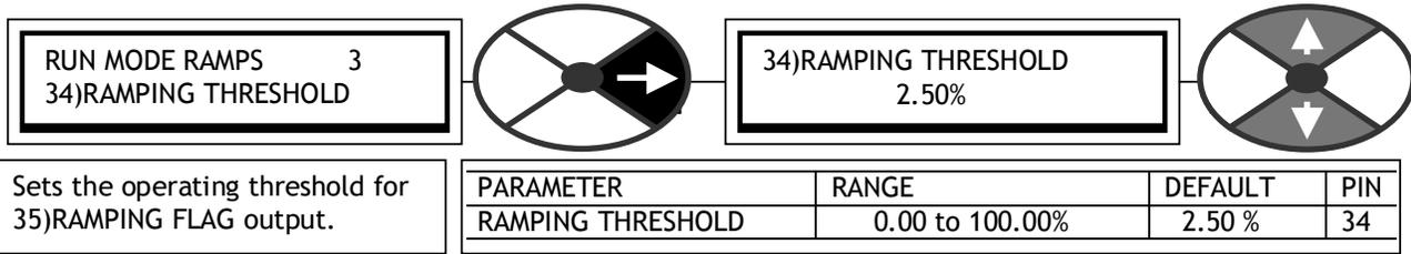
Until the output of the ramp is within this % tolerance of its target value then 35)RAMPING FLAG is high. This is also true if the ramp is being held at a value that differs from the input by more than the threshold. See 6.2.16 RUN MODE RAMPS / Ramping flag PIN 35.
