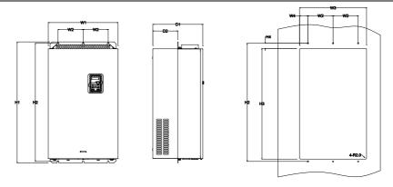
Figure C-15 Flange installation of 660 V 160-220 kW VFDs
