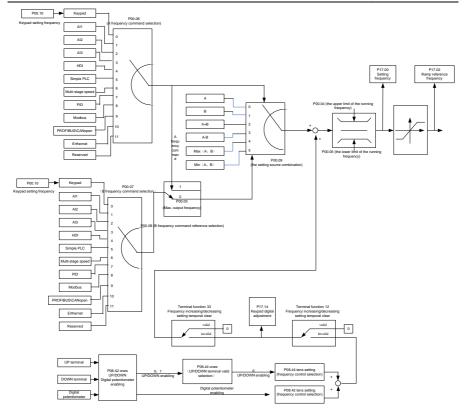
Goodrive35 series VFDs support the shifting between different given channels, and the detailed shifting rules is as below:
