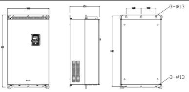
Figure C-5 Wall installation of 380 V 132-200 kW VFDs
