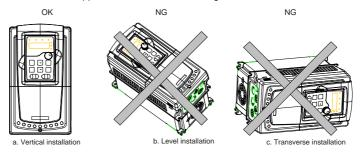
Figure 4-1 Installation direction of the VFD
