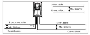
Figure D-3 Wiring layout distances
