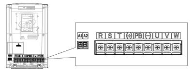
Figure 4-13 Terminals of main circuit for the VFDs of 380 V 22–30 kW
