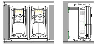
Figure 4-4 Parallel installation
