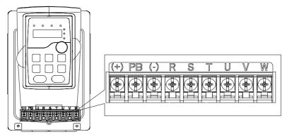
Figure 4-9 Terminals of main circuit for the VFDs of 380 V 1.5-2.2 kW
