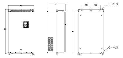
Figure C-12 Wall installation of 660 V 160-220 kW VFDs
