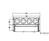
Figure C-16 Floor installation of 660 V 250-350 kW VFDs
