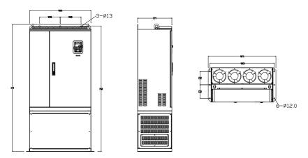
Figure C-10 Floor installation of 380 V 220-315 kW VFDs
