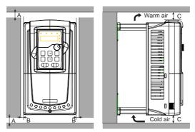
Figure 4-3 Single installation
