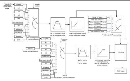
When the user selects the user-defined V/F curve function in Goodrive35 series VFDs, they can set the reference channel of voltage and frequency and the corresponding ACC/DEC time, or the two can be combined to form a real-time curve.
