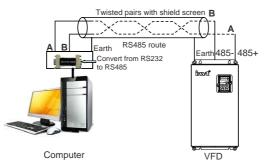
Figure 10-1 RS485 physical connection in single application
