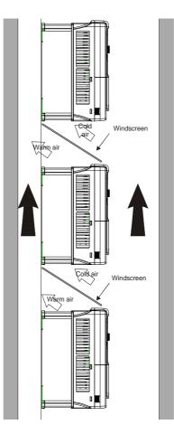
Figure 4-5 Vertical installation
