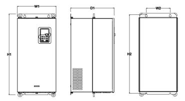
Figure C-11 Wall installation of 660 V 22-132 kW VFDs
