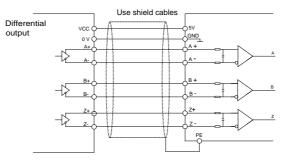
**Note:** The diagram of differential output is given to the H1 interface, C1 interface applies opto-isolator and H2 interface applies differential chips. The external wiring is the same as that of H1.
