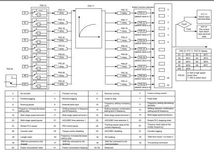
This parameter is used to set the function corresponds to the digital multi-function terminals.
