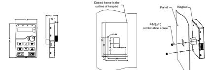
Hole dimension and diagram for keypad installation without bracket
