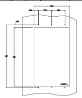
Figure C-9 Flange installation of 380 V 132-200 kW VFDs
