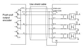
Push-pull output mode wiring diagram 1
