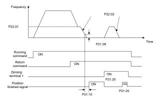
The steps of (1)–(4) are the same as the 4 steps in close-loop vector control mode. The function of spindle positioning is available in the position control mode and speed control mode.
