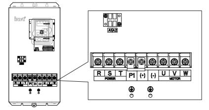
Figure 4-14 Terminals of main circuit for the VFDs of 380 V 37-55 kW and 660 V 22-45 kW
