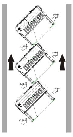
Figure 4-6 Tilt installation
