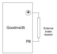
Installation of brake units:
