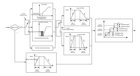
2. The starting logic figure of starting after the restarting function becomes valid during the normal powering on.
