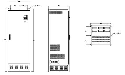
Figure C-17 Floor installation of 660 V 400-630 kW VFDs
